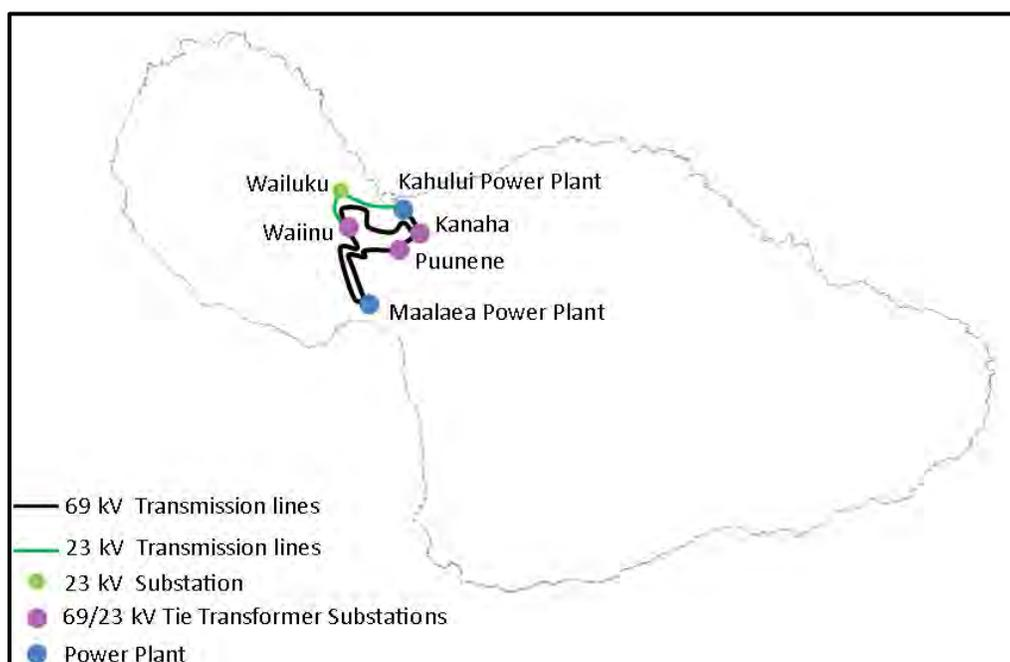
Figure 1: Key central Maui transmission components
