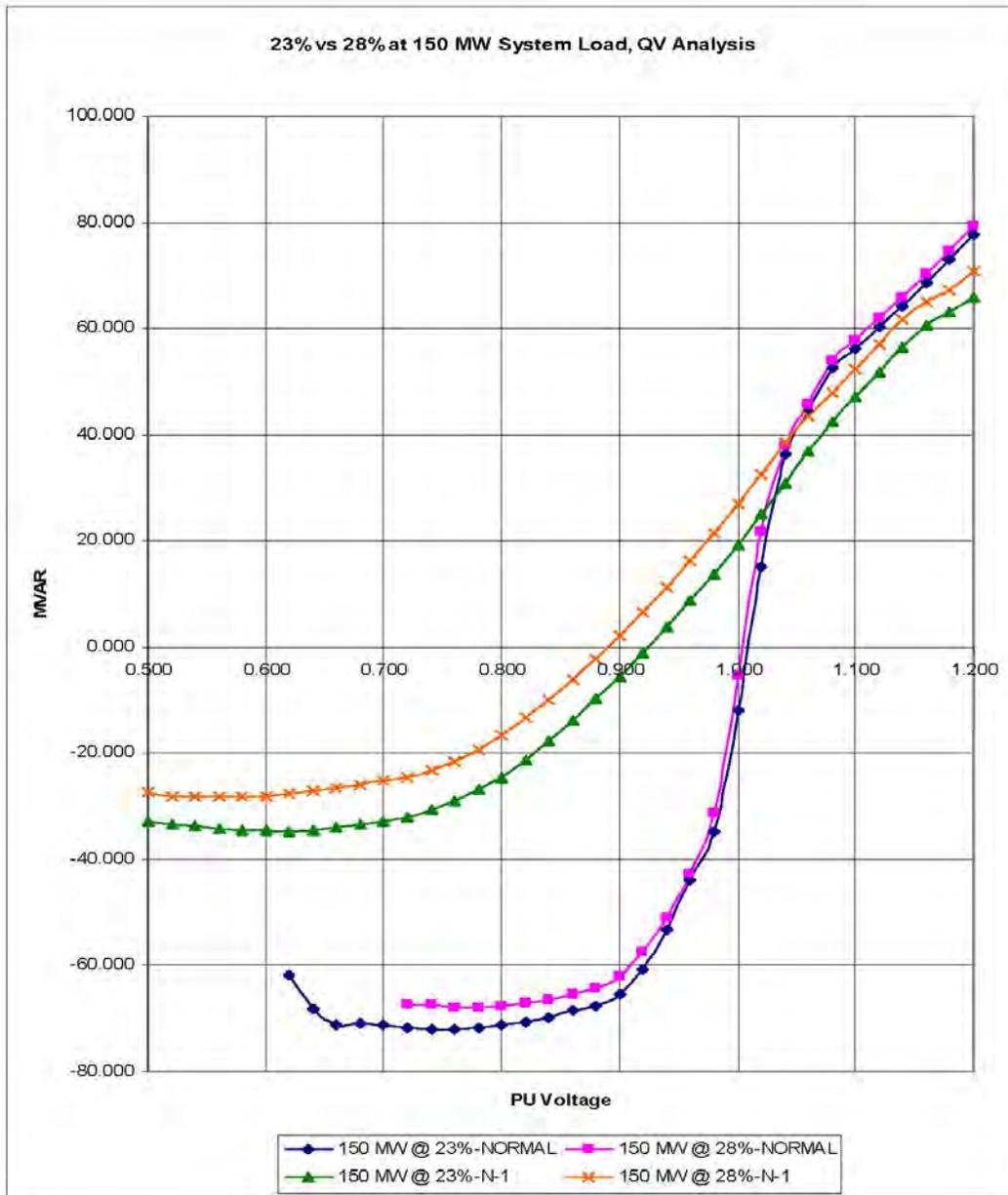
**Figure 7: 23% vs. 28% of 150 MW System Load, QV Analysis**
