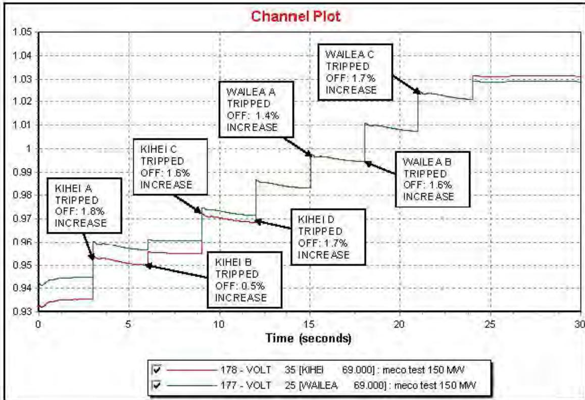
**Figure 10: 150 MW Case Manually Shed Load**
