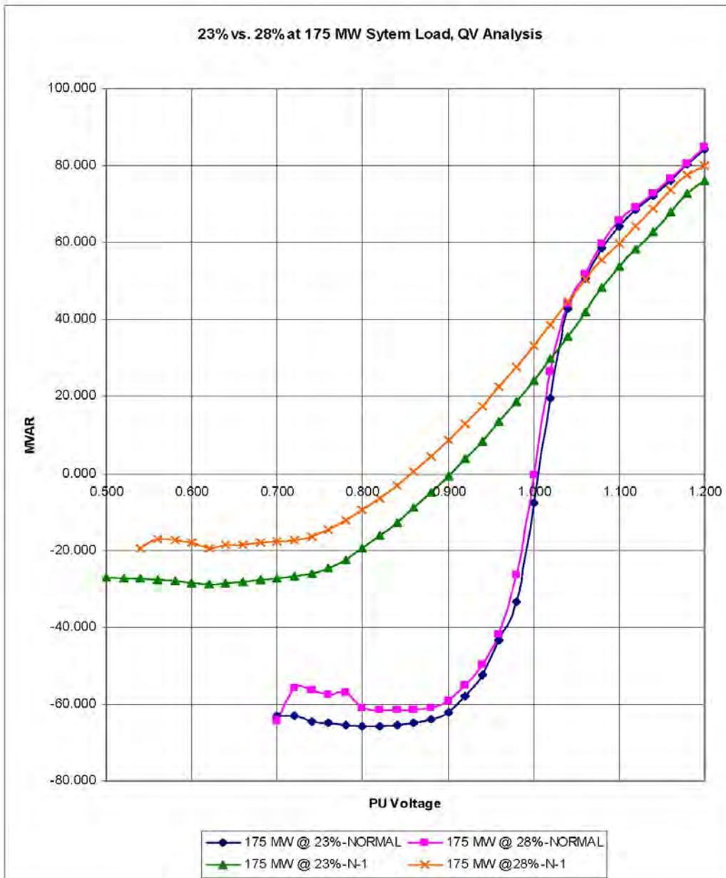
Figure 8: 23% vs. 28% of 175 MW System Load, QV Analysis
