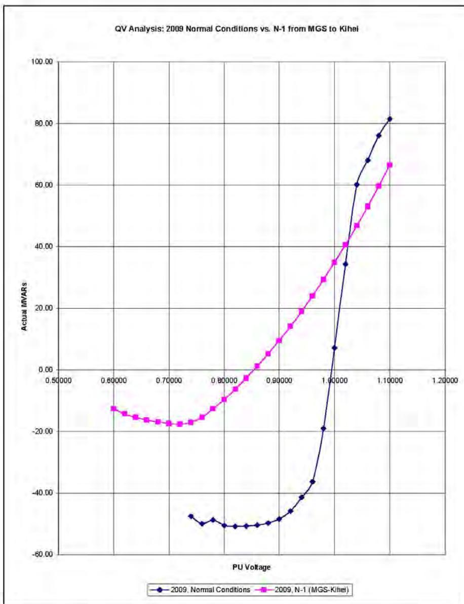
Figure 1: 2009, Normal vs. N-1 (MGS-Kihei) Voltage Collapse Analysis
