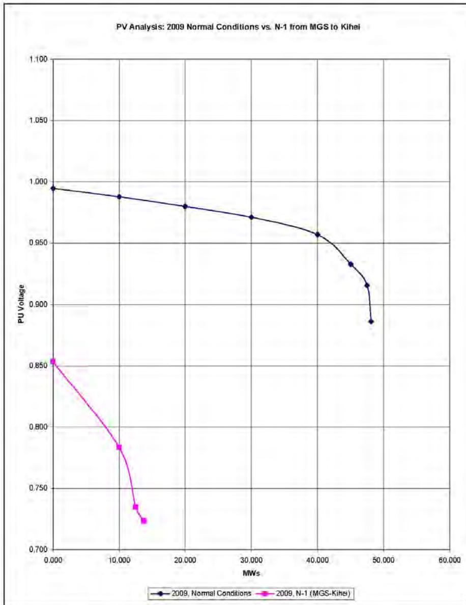
Figure 2: PV Analysis, 2009 Normal Conditions vs. N-1 (MGS-Kihei)
