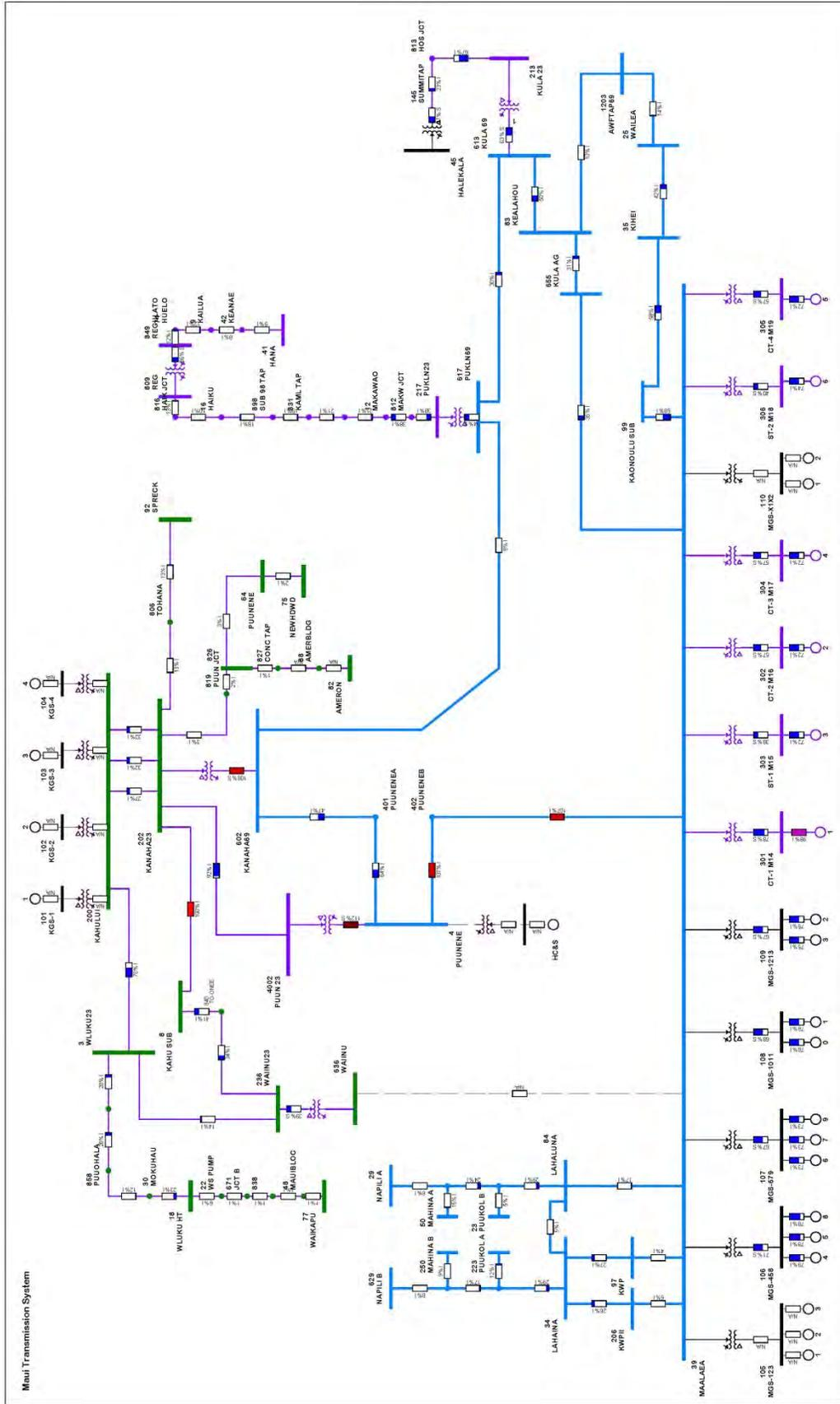
Figure 3: Maui transmission system in 2019 without upgrades under N-1 contingency, loss of MPP-Waiinu
