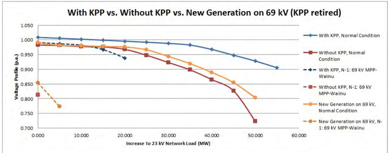
Figure 13: P-V characteristic comparison of the scenario of new generation on the 69 kV network, the existing system with KPP, and the existing system without KPP for the normal condition and most severe N-1 contingency event.
