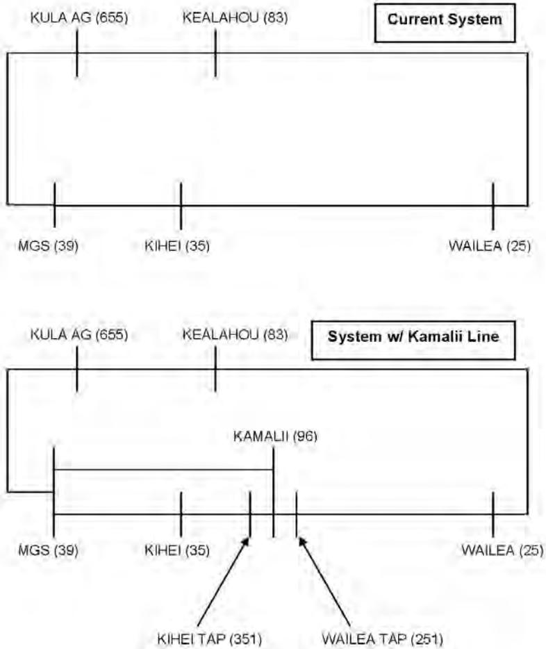
Figure 6: Current System vs. System w/ Kamalii Substation
