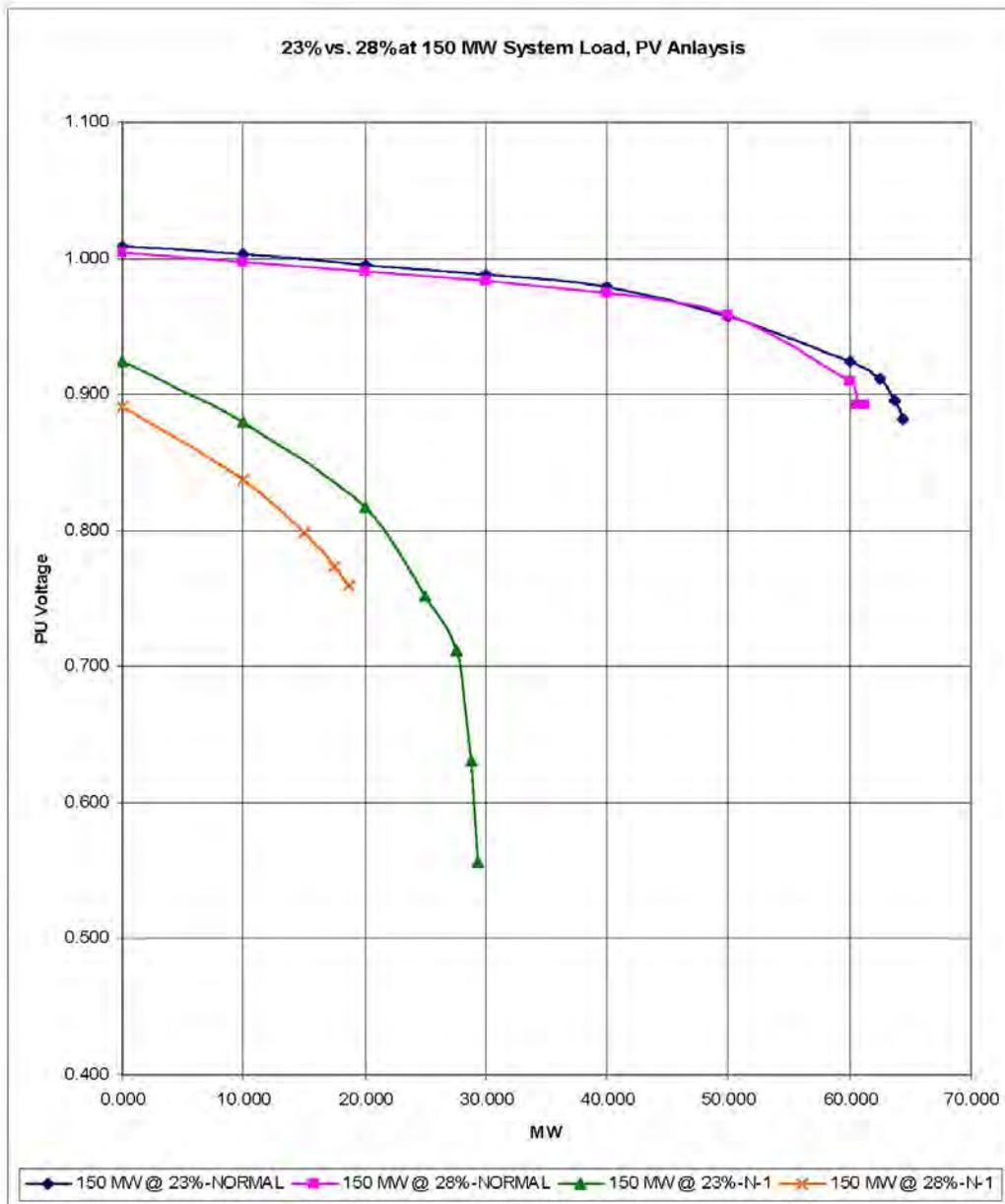
**Figure 5: 23% vs. 28% of 150 MW System Load, PV Analysis**
