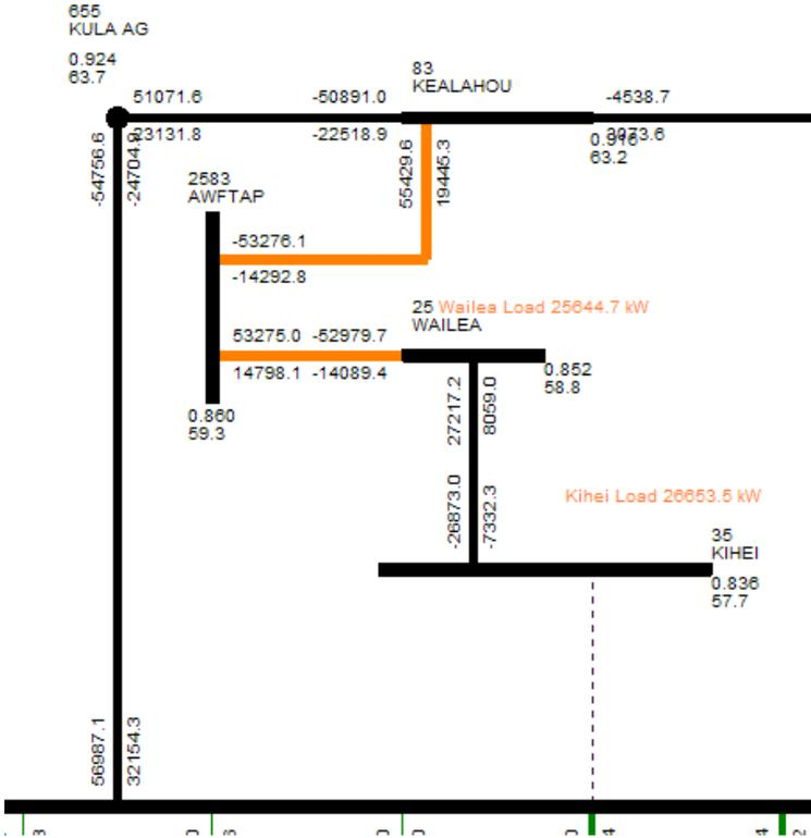
Figure D-I. MPP - Kihei Outage - Boundary Case
