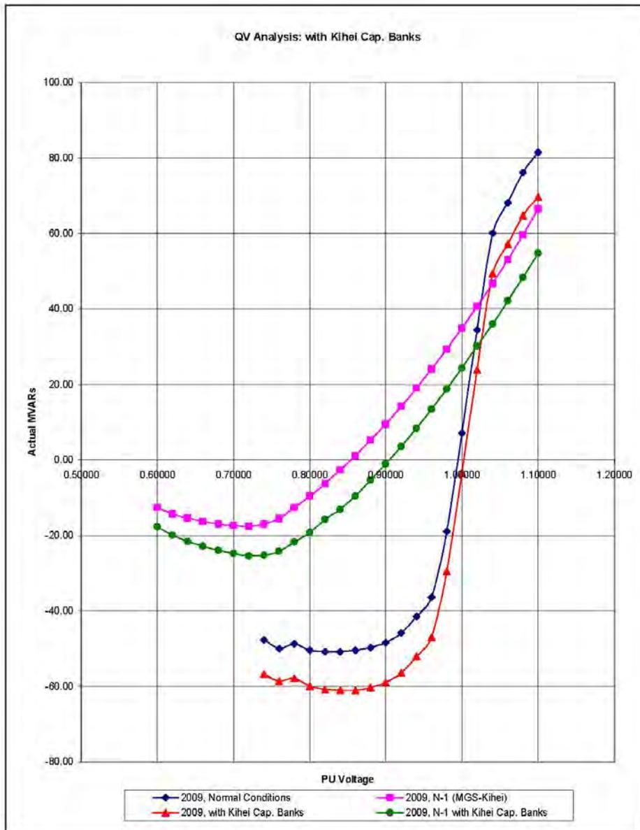
**Figure 5: 2009, with Additional Cap. Banks at Kihei**
