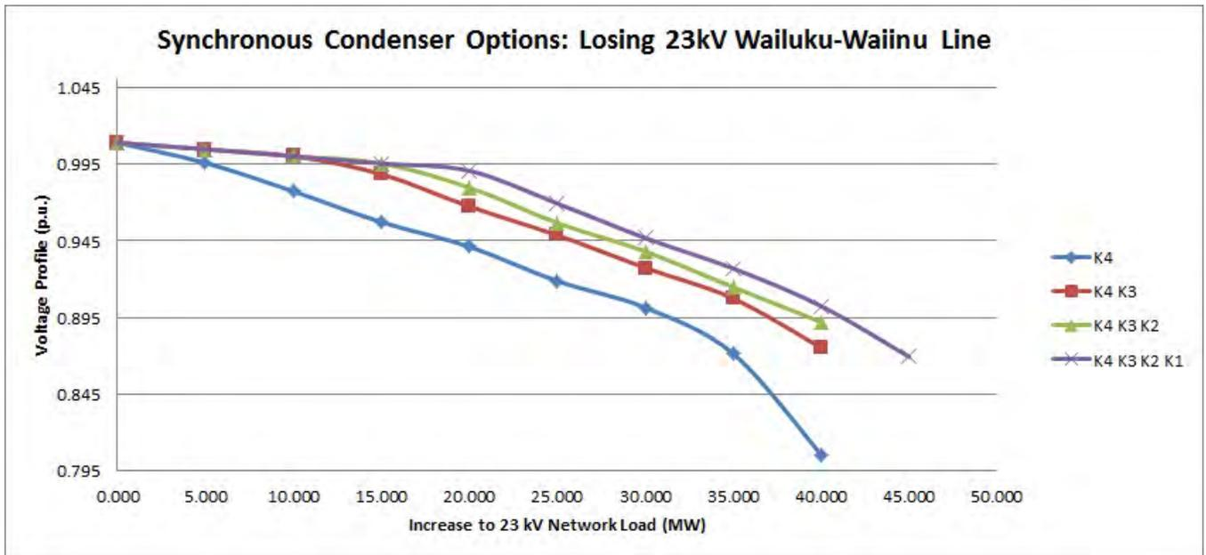
Figure 29: Comparison of P-V characteristics of synchronous condenser options for losing the 23 kV Wailuku-Waiinu Line.
