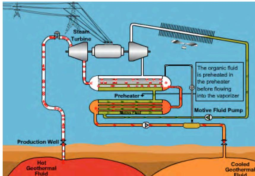
Figure G-12. Geothermal Hybrid Plant
