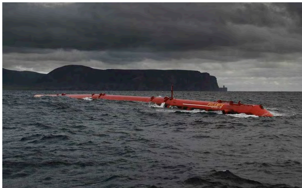
Figure D-76. Pelamix Wave Energy Converter at the European Marine Energy Test Centre (EMEC) 2008
