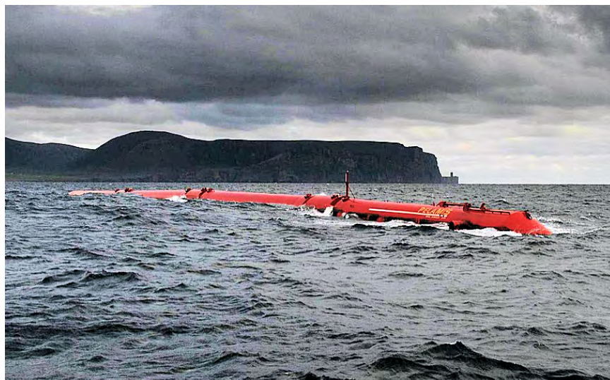
Figure E-2. Pelamix Wave Energy Converter at the European Marine Energy Test Centre, 2008
