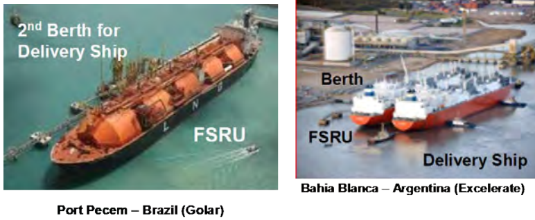
Figure 35: Double Berth and Single Berth Operation
