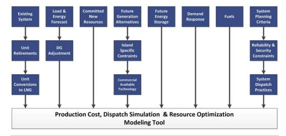
Figure 4-1. PSIP Production Simulation Model Input Hierarchy
