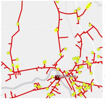
Clicking on an icon reveals detailed information about that installation and the its circuit. Installation information includes its type (solar or wind) and its output capacity; circuit information includes the circuit rating, feeder ID, substation, rating, distributed generation (DG) on the feed, transformer capacity, DG on the transformer, and the remaining capacity in kW and percent of total circuit capacity.
